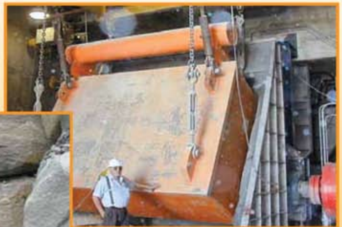
Figure 4 Typical magnetic field configuration of an electromagnet suspended over a conveyor belt. The magnetic field extends outward from the center of the magnet. The magnetic field is strongest at the center and diminishes towards the edges.
